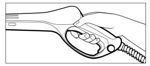
**Step 4** Trigger the gun to eliminate trapped air, wait for a steady flow of water to emerge from the spray nozzle.
